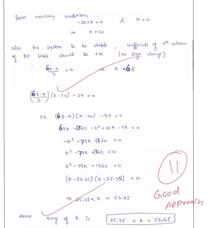
for oscillatory response s' - row conficient =0 =D K = 25.35 08 k = 56-65 putting these values in s2 - vow for k = 25-35 14.252 +25-35 =0 =0 \ w = 1.3 rod/s 14.78 c2 + 53.65 =0 =0 \w = 3.3 rad for k = 53-65
