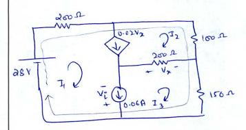
$V_{x} = (I_3 - I_2) 200$ , we'll ux this in other each where each required
