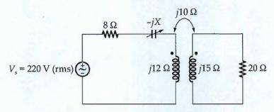
(ii) Calculate current  $I_X$  for the circuit shown below:
