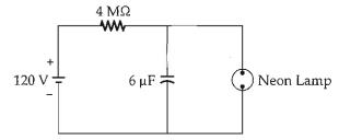
For how long is the lamp on each time the capacitor discharges? What is the time interval between two flashes?
