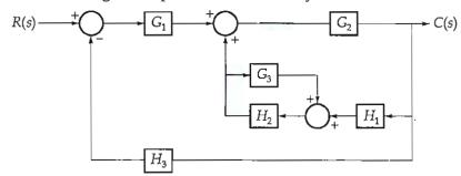
Draw the signal flow graph and determine the overall transfer function using Mason's gain formula.
