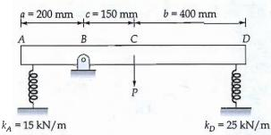
Also, determine the maximum forces resisted by the springs at *A* and *D* and the reaction force at *B*.
