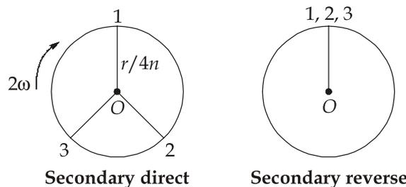
Since secondary direct cranks forms a balanced system and therefore, unbalanced secondary force is due to only secondary reverse cranks and is given by,
