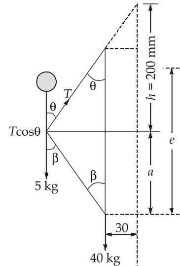
Now, let  $T$  be the tension in upper arms. Considering the vertical component of the forces on the lower link,
