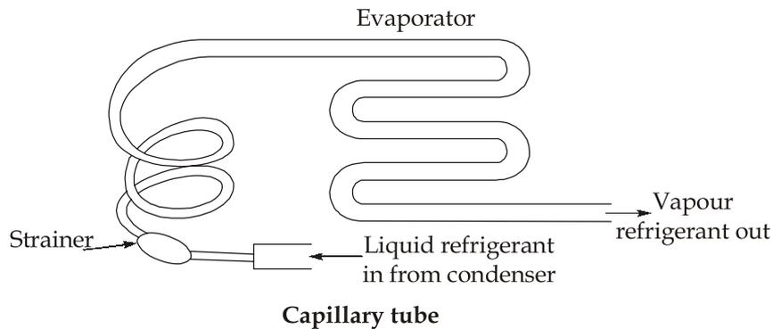
**Advantages of using capillary tube in refrigeration system:**
