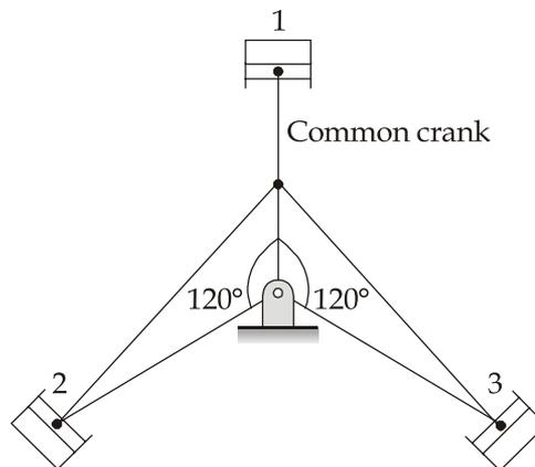
The position of three cylinders is shown in figure.
