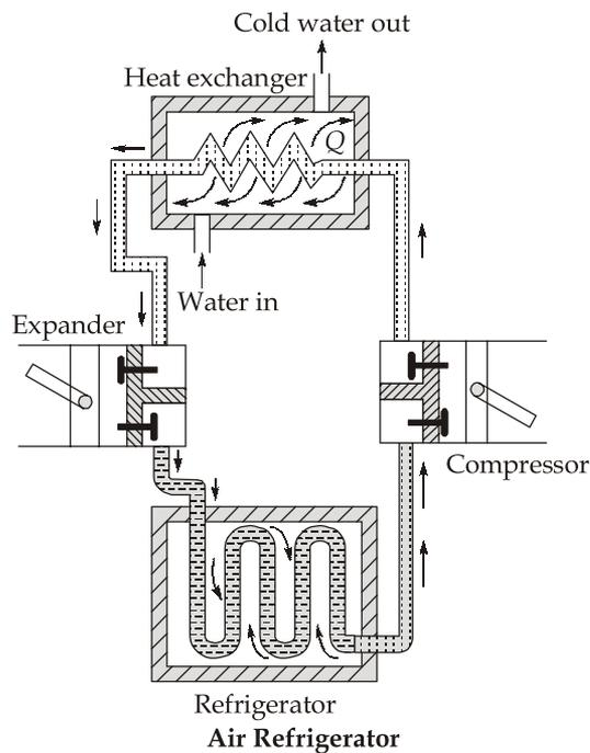
This means that there is reduction in temperature. The temperature of the gas can be reduced by an adiabatic expansion of the gas. This principle was used in the Bell-Coleman air-refrigeration system.
