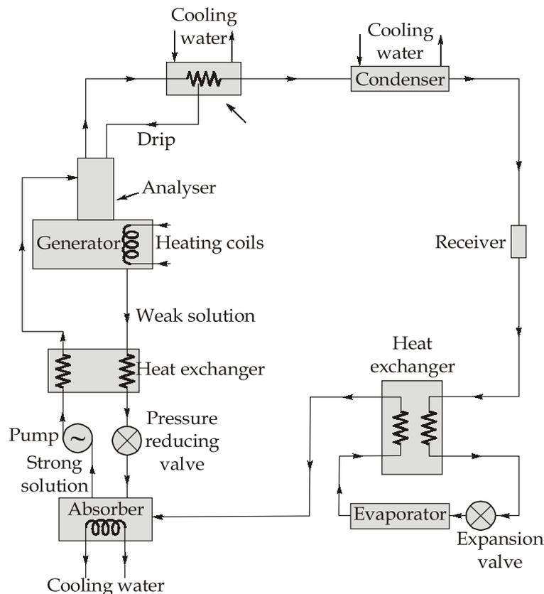
The heat exchanger provided between the condenser and the evaporator may also be called liquid sub-cooler. In this heat exchanger, the liquid refrigerant leaving the condenser is sub-cooled by the low temperature ammonia vapour from the evaporator as shown in figure. This sub-cooled liquid is now passed to the expansion valve and then to the evaporator.
