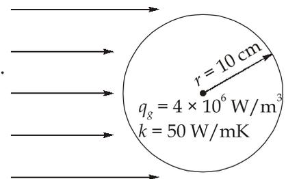
Now, heat generated in the sphere is convected over the surface.
