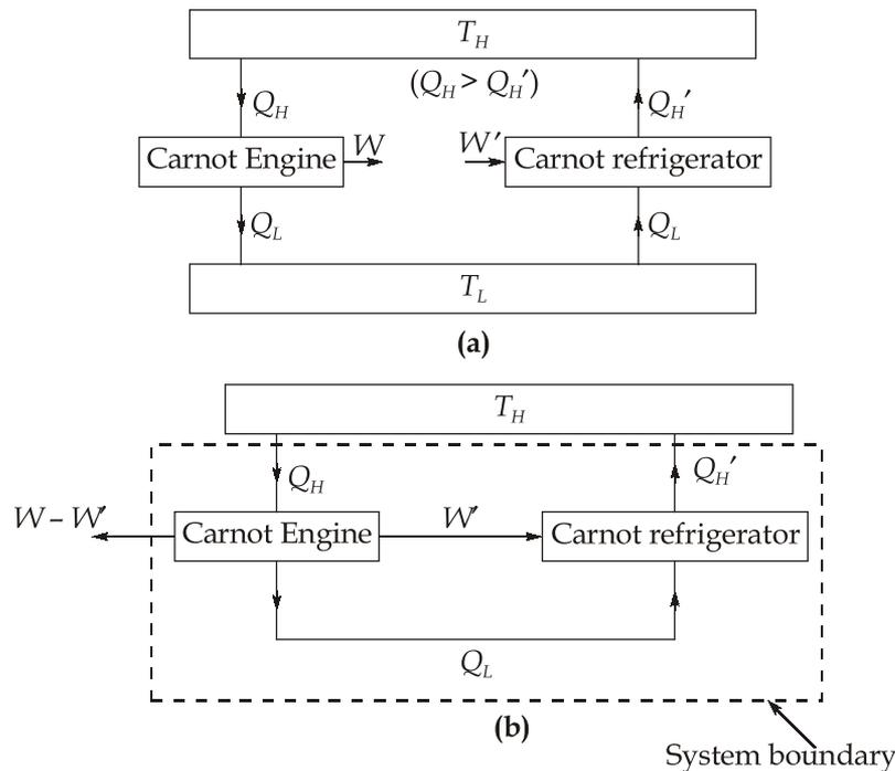
The net result is a heat transfer  $(Q_H - Q'_H)$  from a single reservoir and production of work, which is a clear violation of the second law. Thus, the efficiency of a Carnot engine is not dependent on the working substance.
