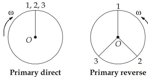
Since primary reverse cranks form a balanced system and therefore, unbalanced primary force is due to direct cranks only and is given by,
