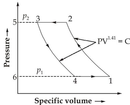
We have  $\frac{T_2}{T_1} = \frac{T_3}{T_4} = \left( \frac{P_2}{P_1} \right)^\gamma = \left( \frac{5}{1} \right)^{1.41} = 1.5968$
