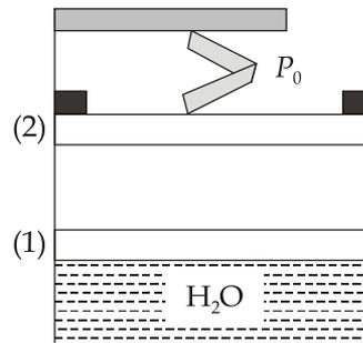
Given:  $m_w = 1$  kg (Saturated),  $P_0 = 100$  kPa,  $P_1 = 100$  kPa,  $V_1 = 0.2$  m<sup>3</sup>,  $V_2 = 1$  m<sup>3</sup>
