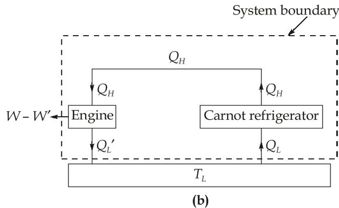
The engine drives the refrigerator using the heat rejected from the refrigerator. But there is some net work ( $W - W'$ ) that leaves the system.
