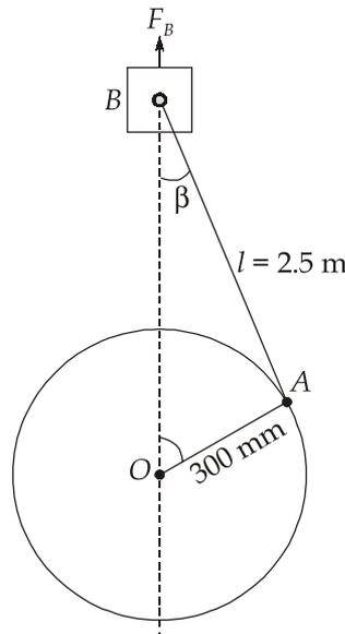
Mass at the crank pin,  $m_a = 220 \times \left( \frac{2.5 - 1}{2.5} \right) = 132 \text{ kg}$
