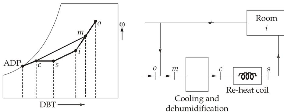
Room air at state  $i$  mixes with ventilation air from surroundings at  $o$  and then enters cooling and dehumidification coil at state  $m$ . Exit happens at  $c$  post which it enters re-heat coil to achieve delivery temperature  $t_s$ .
