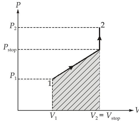
$$W_{CV} = \frac{(P_1 + P_{stop})}{2} (V_{stop} - V_1)$$
