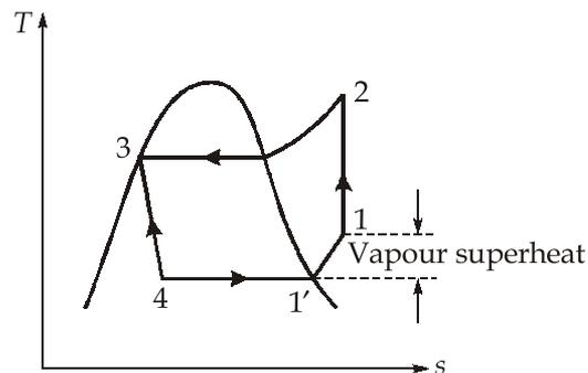
In this case heat from motor winding is continuously heating to suction vapour which passes over it in the refrigeration circuit. This raises the temperature of suction vapour as motor cooling load also becomes a part of the overall cooling load of refrigeration system. Hence, suction vapour which enters at a saturated condition to the compressor gets heated by motor winding and always becomes super heated.
