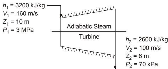
Applying Steady Flow Energy Equation (SFEE)
