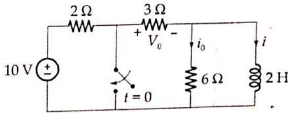
Find  $i_0$ ,  $V_0$  and  $i$  for all time, assuming that the switch was open for a long time. [10 marks]
