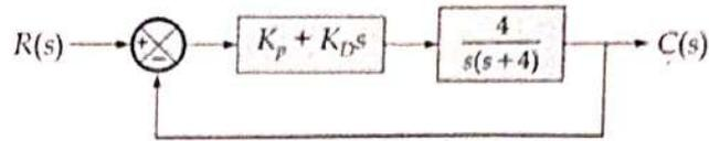
Determine the value of  $K_p$  and  $K_D$  such that the damping ratio of the system will be 0.75 and the steady state error for unit ramp input will be 0.20.
