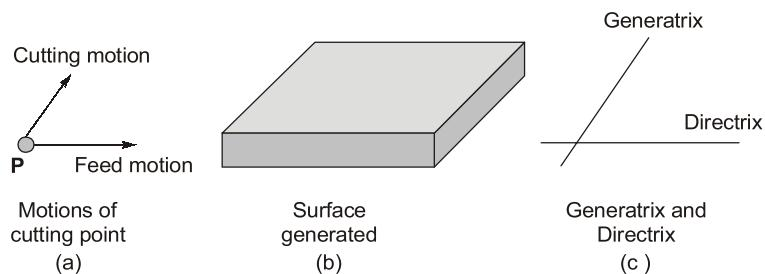
So, various shapes can be obtained depending on the shapes of generatrix and directrix and their relative motion.
