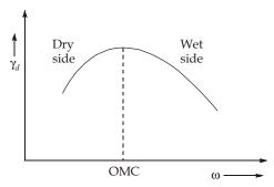
On dry side of OMC, for a given compactive effort, the permeability decreases with increase in water content. The minimum permeability reaches at maximum dry density at OMC.
