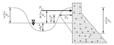
The force due to wave action  $(P_w)$  acts at a distance  $\frac{3h_w}{8}$  above the reservoir surface.
