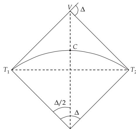
$$\begin{aligned}\text{Apex distance } (V_c) &= R \left( \sec\left(\frac{\Delta}{2}\right) - 1 \right) \\ &= 215 \left( \sec\left(\frac{60^\circ}{2}\right) - 1 \right) = 33.26 \text{ m}\end{aligned}$$
