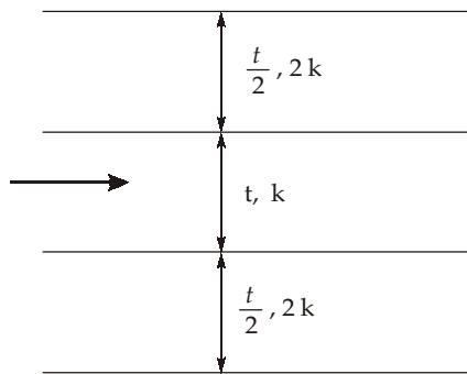
$$k_H = \frac{\sum k_i z_i}{\sum z_i} = \frac{2k \times (t/2) + k \times t + 2k \times (t/2)}{(t/2) + t + (t/2)} = 1.5 \text{ k}$$
