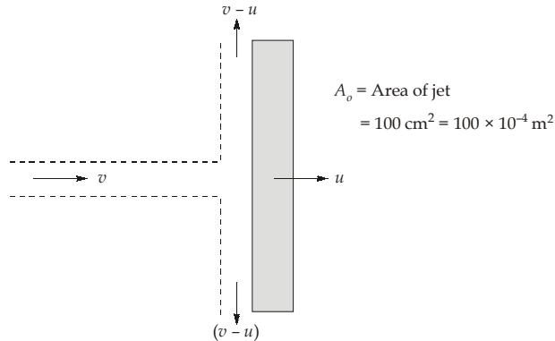
The force exerted by the jet in the direction normal to the plate is given by
