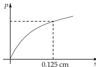
Modulus of subgrade reaction is calculated corresponding to the settlement of 0.125 cm.
