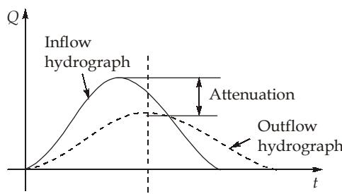
peak of flood hydrograph is lowered and its time base is lengthened.
