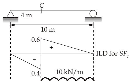
$$\text{Maximum shear force in the beam} = \frac{1}{2} \times 0.6 \times 6 \times 10 = 18 \text{ kN}$$
