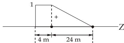
So, maximum shear force at section H is given as
