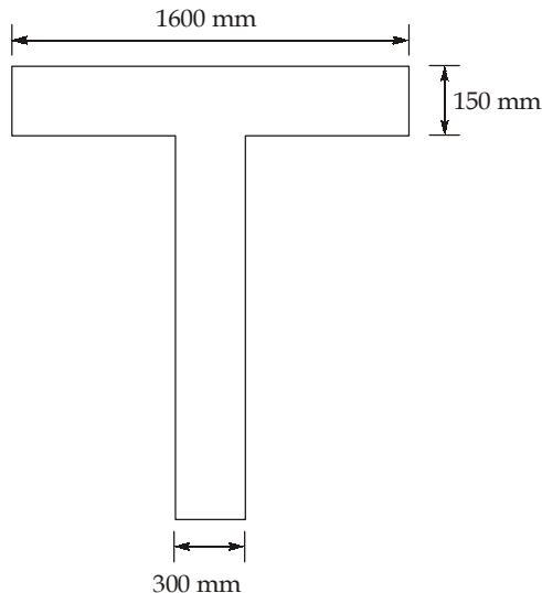
As per IS 456: 2000 clause 23.1.2. For continuous beam;  $l_o$  may be assumed as 0.7 times the effective span.
