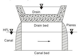
A super passage is reverse of an aqueduct. A super passage is constructed where the bed of drain is well above the canal FSL and canal flows at atmospheric pressure under the bed of drain.
