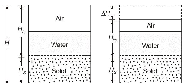
*Fig.* Settling compaction
