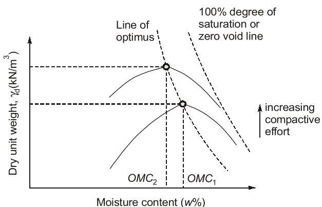
Fig. Compaction Curve
