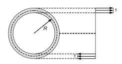
The shear stress distribution is assumed uniform across the thickness and is given by
