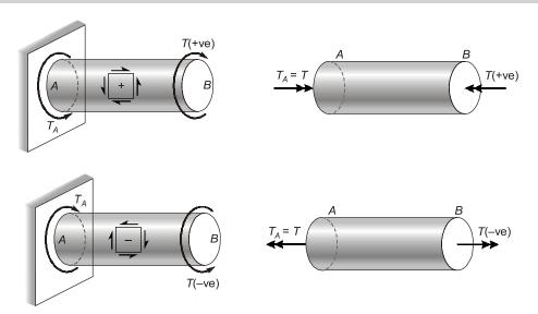
The sign convention can be explained with the help of right hand thumb rule. If torque is applied in the direction of right hand finger, the movement of nut due to torque will be in the direction of right hand thumb. If right hand thumb pointed towards cross-section, then torque is treated positive at that section. A positive torque will produce positive shear stress element on the surface and vice-versa.
