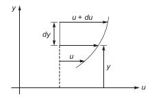
• Upper layer which is moving faster tries to draw the lower slowly moving layer along with it. Similarly, as a reaction to this, the lower layer tries to retard the upper one. Thus there exists a shear between the two layers as shown below.
