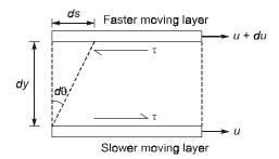
• In time dt, the top layer will move with respect to the bottom layer by a distance  $ds = du \cdot dt$ .
