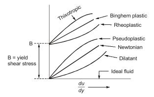
Example-1.3 The Rheological diagram depicting the relation between shear stress and strain rate for different types of fluids is shown in figure below.
