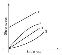
The most suitable relation for flow of toothpaste being squeezed out of the tube is given by the curve:
