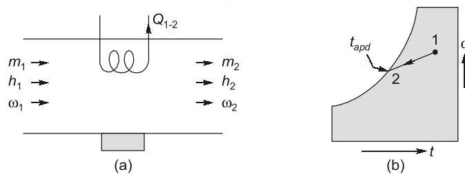
(a) Schematic device of cooling and dehumidification (b) Boiling and dehumidification
