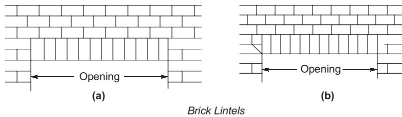
The depth of brick lintel varies from 10 to 20 cm, depending upon the span.
