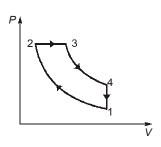
$$\eta_2 = 1 - \frac{1}{r^{\gamma - 1}} \left[ \frac{r_{c_2}^{\gamma} - 1}{\gamma(r_{c_2} - 1)} \right] = 1 - \frac{1}{(12)^{0.4}} \left[ \frac{8^{1.4} - 1}{1.4(8 - 1)} \right] = 0.343$$
