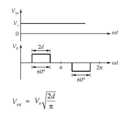
$$V_{0 \text{ rms}} = 300 \sqrt{\frac{60^{\circ}}{180^{\circ}}} = 173.20 \text{ V}$$
