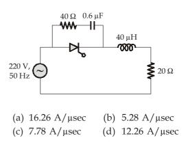
Q.20 In the circuit shown below, the maximum value of current which passes through inductor will be
