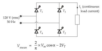
Where,  $V_m$  is peak sinusoidal value,  $\alpha$  is firing angle and  $V_T$  is thyristor voltage drop For  $V_m = 120\sqrt{2} V_T$
