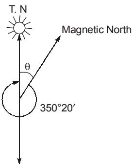
$\therefore$  Magnetic declination,  $\theta = 360^\circ - 350^\circ 20' = 9^\circ 40'$
