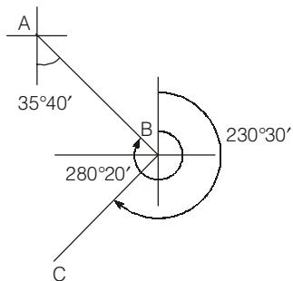
Interior angle =  $280^\circ 20' - 230^\circ 30' = 49^\circ 50'$
