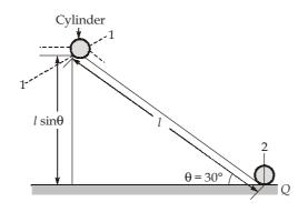
Cylinder rolls without slipping with angular speed  $\omega = \frac{v}{r}$  about its axis.
