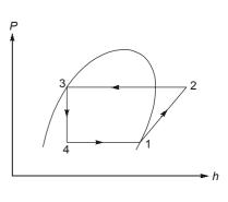
Power consumption =  $\dot{m}(h_2 - h_1) = 0.3652 (215 - 190) = 9.13 \text{ kW}$
