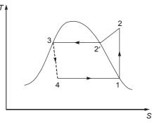
Enthalpy at discharge,  $h_2 = h_{2'} + c_P(T_2 - T_{2'})$
