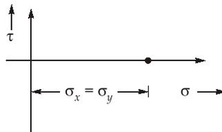
Ex. Hydrostatic pressure, internal contact pressure in hollow shafts due to press-fitting of bearing.
