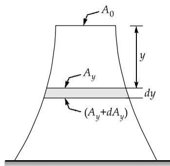
Let us consider a cross-sectional area  $A_y$  at a distance  $x$  from top and having thickness  $dy$  (as shown)
