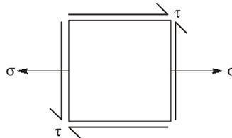
State of stress,  $\sigma = \frac{P}{2\pi r t}$  (Area of cross-section for a thin tube =  $2\pi r t = \pi d t$ )
