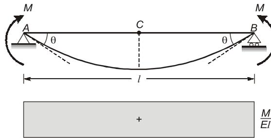
$$\theta_C - \theta_A = \text{Area of } \frac{M}{EI} \text{ diagram}$$
