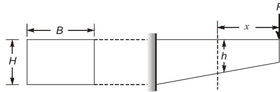
$$\text{Stress at support, } \sigma_1 = \frac{M}{Z} = \frac{P \times L}{\left(\frac{B \times H^3}{12}\right)} \times \frac{H}{2} = \frac{6PL}{BH^2}$$
