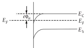
When a positive voltage is applied to the semiconductor, (i.e., reverse bias), the energy band diagram is as below:
