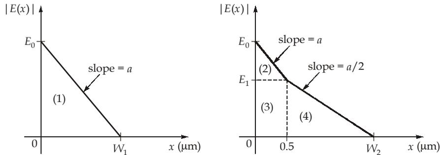
When  $E_0 =$  critical electric field  $= 4 \times 10^5 \text{ V/cm}$ , the area under the plot of  $|E(x)|$  is equal to the breakdown voltage.
