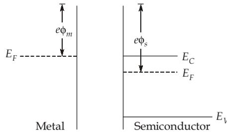
When they come in contact, to achieve thermal equilibrium in the junction, electrons flow from the metal into the lower energy states in the semiconductor, which makes the surface of the semiconductor more *n*-type. The excess charge in the *n*-type semiconductor exists essentially as a surface charge density.
