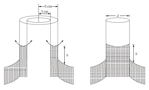
For fluid rise between 2 concentric capillary tubes, we know that,
