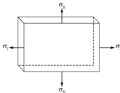
For this condition,  $\tau_{\max} = \max \left\{ \frac{\sigma_h}{2}, \frac{\sigma_l}{2}, \frac{\sigma_h - \sigma_l}{2} \right\} = \frac{pd}{4t}$
