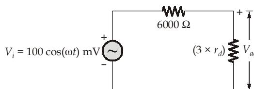
$$r_d = \frac{V_T}{I_D} = \frac{25 \text{ mV}}{1 \text{ mA}} = 25 \Omega$$
