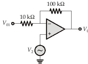
There are two inputs  $V_{01}$  and  $V_2$ , so by applying superposition theorem.
