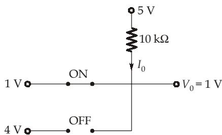
$$I_0 = \frac{5V - V_0}{10\text{k}\Omega} = \frac{5V - 1V}{10\text{k}\Omega} = 0.4 \text{ mA}$$
