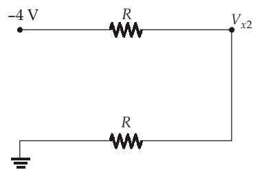
$$V_{x2} = (-4) \times \frac{R}{2R} = -2V$$
