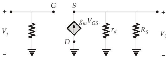
$$V_0 = g_m V_{GS} (r_d || R_s)$$
