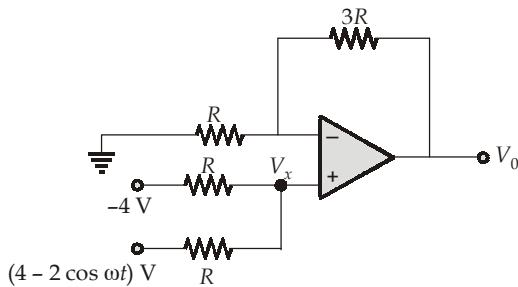
$$V_0 = \left[ 1 + \frac{3R}{R} \right] V_x = 4V_x \quad \dots(i)$$
