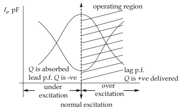
Feeds lagging KVAR to the bus but absorbs the leading kVAR.
