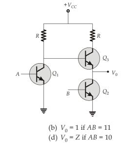
(a)  $V_0 = 0$  if AB = 00(c)  $V_0 = 1$  if AB = 10
