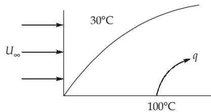
$$\begin{aligned} \text{Reynold number, } Re_L &= \frac{U_\infty L}{\nu} = \frac{30 \times L}{18.97 \times 10^{-6}} \\ &= 1.5814 \times 10^6 L \end{aligned}$$
