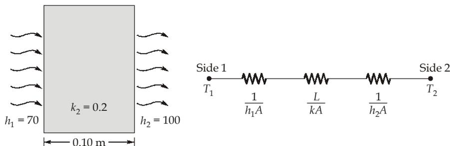
$$\begin{aligned} T_1 - T_2 &= Q \times R = 100 \times 0.5242 \\ &= 52.42^\circ\text{C} \approx 52.4^\circ\text{C} \end{aligned}$$
