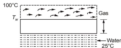
$$\text{Rate of heat transfer} = \frac{T_g - T_w}{\Sigma R}$$
