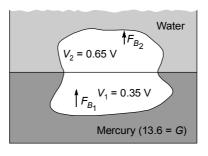
Buoyancy force due to mercury
