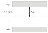
$$\therefore \qquad \text{shear stress, } \tau = \mu \frac{du}{dy}$$
