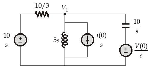
$$\frac{\left(V_1 - \frac{10}{s}\right)}{\frac{10}{3}} + \frac{V_1}{5s} - \frac{1}{s} + \frac{\left(V_1 - \frac{5}{s}\right)}{\left(\frac{10}{s}\right)} = 0$$
