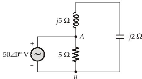
$$V'_{AB} = 50\angle 0^\circ + 0 \text{ V} = 50\angle 0^\circ \text{ V}$$
