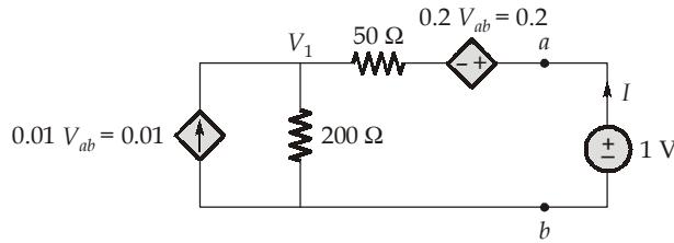
$$0.01 = \frac{V_1}{200} + \frac{V_1 - 1 + 0.2}{50}$$
