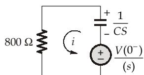
$$v(t=2 \text{ ms}) = 50 e^{\frac{-2 \times 10^{-3}}{800 \times 2 \times 10^{-6}}} = 14.33 \text{ V}$$
