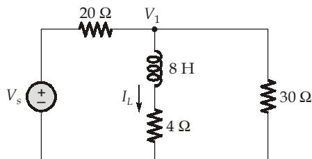
$$\frac{(V_1 - V_s)}{20} + \frac{V_1}{8s + 4} + \frac{V_1}{30} = 0$$
