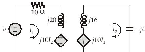
$$-60\angle 30^\circ + (10 + 20j)I_1 + j10I_2 = 0 \quad \dots(i)$$
