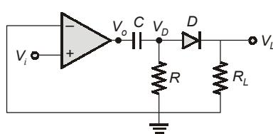
The op-amp will work as a zero crossing detector, thus the output at node  $V_o$  is equal to
