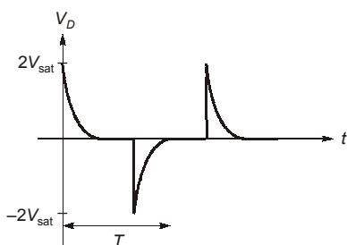
Now, at last state the diode circuit will acts as a negative clipper and the output waveform will look like
