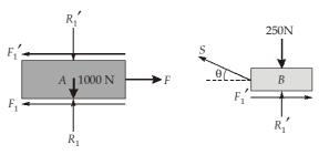
$$F_1 = \mu R_1 \text{ and } F_1' = \mu R_1'$$
