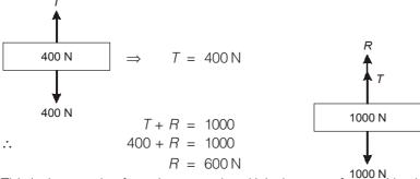
This is the reaction from the ground and it is the same force with which the 1000 N block press against the floor.
