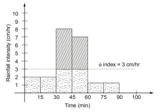
Hatched portion shows the total runoff and dotted portion shows the total infiltration.
