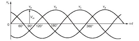
$V_A = V_m \sin \omega t$ Phase *A* will get maximum voltage at  $\omega t = 90^\circ$ . At this instant
