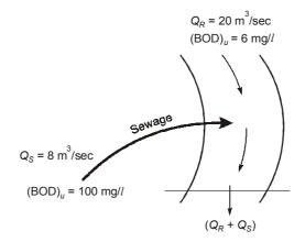
Given, Cross section area of river =  $80 \text{ m}^2$
