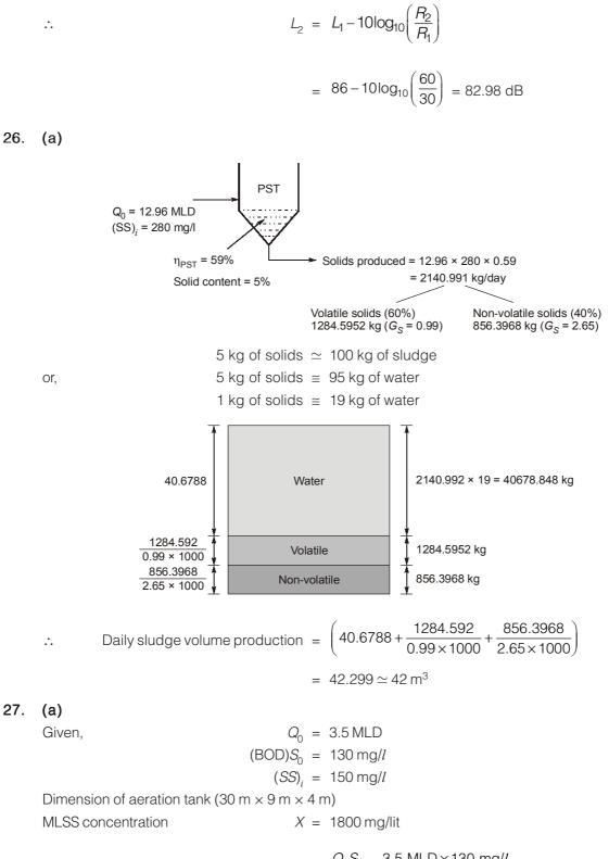
$\therefore \qquad \text{BOD loading rate} = \frac{Q_0 S_0}{V} = \frac{3.5 \text{ MLD} \times 130 \text{ mg/}l}{\left(\frac{30 \times 9 \times 4}{10^4}\right) \text{ha-m}}$ = 4212.96 kg/ha-m/day
