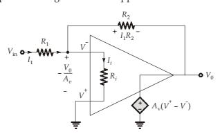
$$V_{0} = -\frac{R_{2}}{R_{1}} \left[ V_{\text{in}} + \frac{V_{0}}{A_{v}} \right] - \frac{V_{0}}{A_{v}}$$
