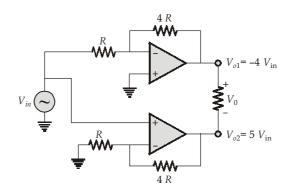
$$\begin{array}{lll} \ddots & & & & & \\ V_o & = & V_{o_1} - V_{o_2} & & \\ & = & -4 \ V_{\rm in} - 5 \ V_{\rm in} \\ & = & -9 \ V_{\rm in} \\ \end{array}$$
