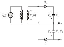
The circuit represents a voltage doubler circuit, if the voltage was taken by adding voltages of both the capacitors, but to calculate  $V_0$  we have to find the voltage stored on a single capacitor. Thus, comparing from the above figure,
