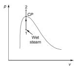
Constant volume heat addition process passing through critical point.
