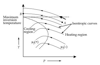
As gas is throttled above maximum inversion temperature (curve AB and above) then the temperature of gas keeps on increasing.
