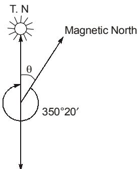
$$\therefore \text{Magnetic declination, } \theta = 360^\circ - 350^\circ 20' = 9^\circ 40'E$$
