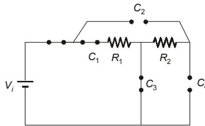
Series combination of  $C_2$  and  $C_4$  is connected across  $V_i$  directly. So  $C_2$  and  $C_4$  will charge instantly.
