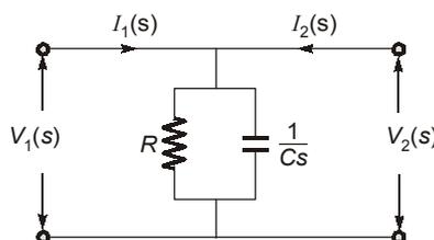
$$V_2(s) = I_1(s) \left( \frac{R \times \frac{1}{Cs}}{R + \frac{1}{Cs}} \right)$$
