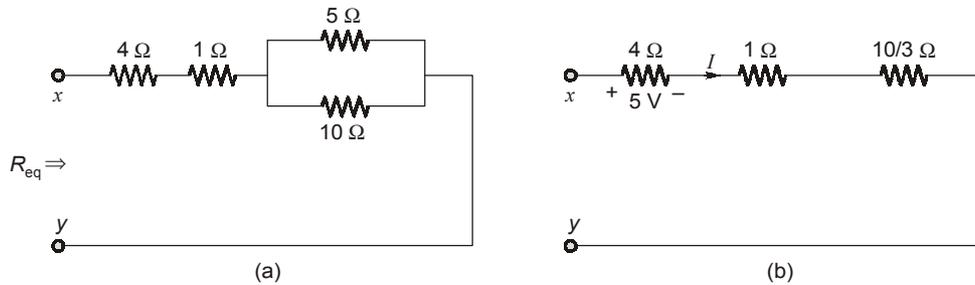
$$\begin{aligned} R_{\text{eq}} &= 4 \Omega + 1 \Omega + (5 \parallel 10) \Omega \\ &= 5 \Omega + \left( \frac{5 \times 10}{15} \right) \Omega \\ &= 5 + \frac{10}{3} = \frac{25}{3} \Omega \end{aligned}$$
