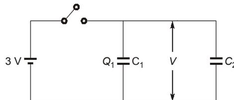
Let Charge stored in  $C_1 = Q_1$ Charge stored in  $C_2 = Q_2$
