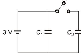
$C_1$  gets charged upto 3 V charge stored in  $C_1$
