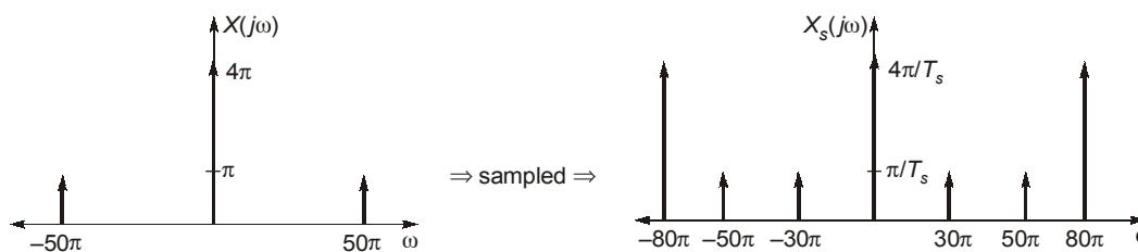
$$X_s(j\omega) = 40 \sum_{m=-\infty}^{\infty} [4\pi\delta(\omega - 80\pi) + \pi\delta(\omega - 50\pi - 80\pi m) - \pi\delta(\omega + 50\pi - 80\pi m)]$$
