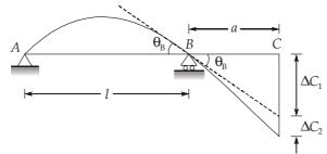
Now  $\Delta C_1$  is produced due to deflection of *C* as caused due to deformation of *AB*,  $\Delta C_1 = \theta_B (BC) = \theta_B a$
