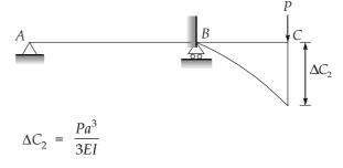
So total deflection at  $C_{,\Delta}C = \Delta C_{1} + \Delta C_{2}$
