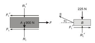
$$F_1 = \mu R_1 \text{ and } F_1' = \mu R_1'$$
