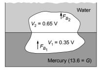
Buoyancy force due to mercury
