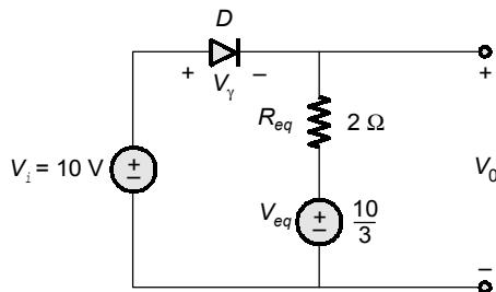
$$V_{eq} = \frac{-\frac{10}{6} + \frac{10}{3}}{\frac{1}{6} + \frac{1}{3}} = \frac{10 \times \frac{3}{18}}{\frac{9}{18}} = \frac{10 \times 3}{9} = \frac{10}{3} \text{ volts.}$$
