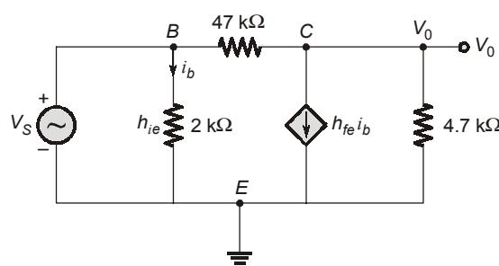
$$i_b = \frac{V_s}{h_{ie}} = \frac{V_s}{2 \text{ k}\Omega}$$
