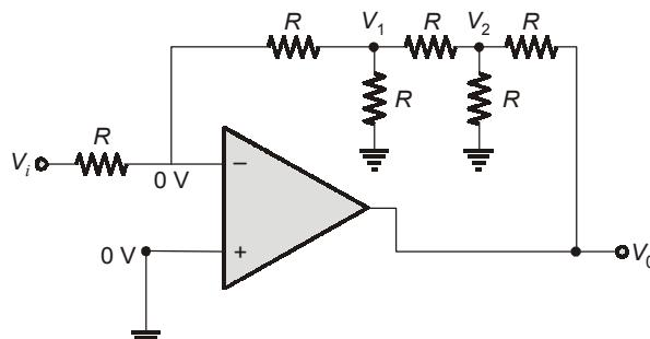
$$\frac{3V_1}{R} = \frac{V_2}{R}$$
