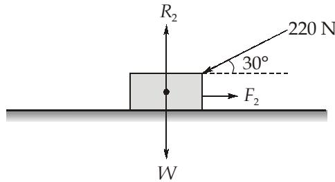
$$\begin{aligned} R_2 &= W + P_1 \sin 30^\circ = (W + 220 \times 0.5) \\ &= (W + 110) \text{ N} \end{aligned}$$
