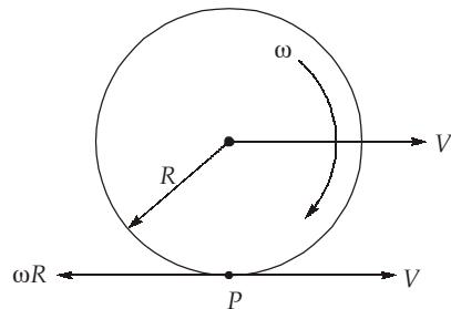
$$\text{Net velocity at } P (V_p) = V - \omega R = 0 (\therefore \text{In pure rolling } V = \omega R)$$
