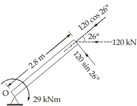
$$\begin{aligned}M_o &= 120 \sin 26^\circ \times 2.8 \text{ (ACW)} - 29 \text{ (CW)} \\&= 118.2927 \text{ kNm (ACW)}\end{aligned}$$
