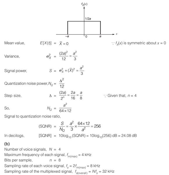
Overall transmission rate,  $R_b = nf_{s(overall)} = 256$  kbps
