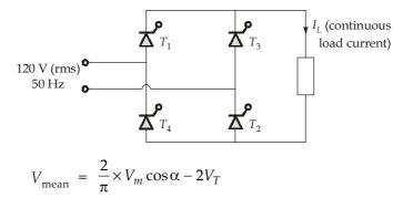
Where,  $V_m$  is peak sinusoidal value,  $\alpha$  is firing angle and  $V_T$  is thyristor voltage drop
