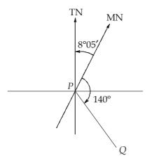
True bearing of PQ = Magnetic bearing ± magnetic declination E/W
