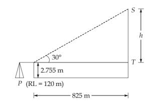
RL of top of tower = Height of instrument at P + h= (120 + 2.755) + 825 tan 30° = 599.07 m
